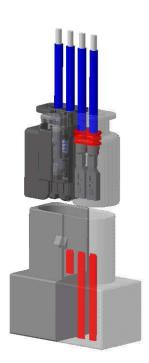
The plug–in connection is completed by inserting vertically in a suitable unit connection or pin housing until the clip is correctly engaged. Engaging of connector housing in counterpart is ensured by clicking. After a correct connection the CPA can be engaged with is also ensured by clicking.
