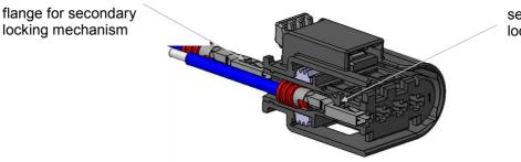
secondary locking mechanism latch
