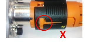
If the connector is not at the final position – the locking hook stays outside – a movement of the CPA (black part) is not possible.
