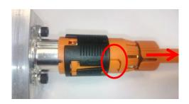
Pressing area of locking hook on both sides. If it is easier, it is allowed to support by pulling at the cable.
