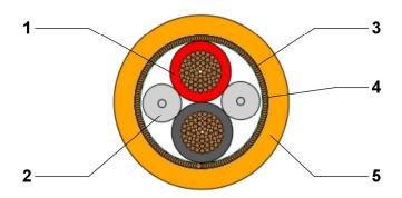
1. 2 Cores 4.0 mm<sup>2</sup> Type RADOX 155S FLR-B
