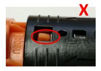
If the connector is not in the final position – the locking hook stays outside – a movement of the CPA (black part) is not possible.
