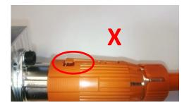
If the connector is not at the final position – the locking hook stays outside.
